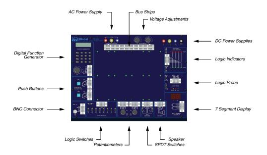
Figure 1 PB-505A Components
