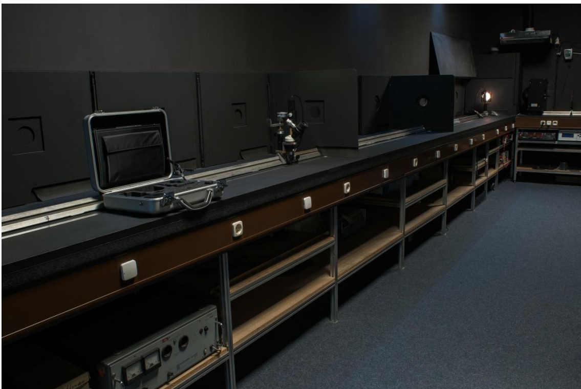
GOSSEN Light Lab – Optical Table for the Calibration of Illuminance and Luminance
