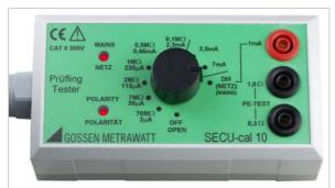
All limit values for the required tests per DIN VDE, as well as protective conductor resistance, insulation resistance, equivalent leakage current, differential and/or contact as well as housing leakage current must be tested.
