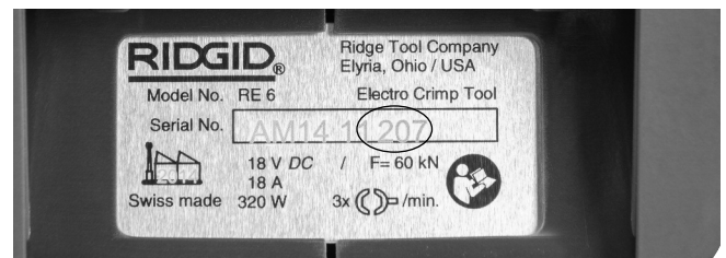
Figure 3 – Machine Serial Number - The first 4 digits (circled) indicate the year and month of manufacture. (12 = year, 06 = month).
