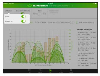
Additionally, parabolas are shown that display the different Wi-Fi networks in that area in terms of frequency occupancy/channel and strength, with the option of viewing either 2.4 GHz or 5 GHz bands.
