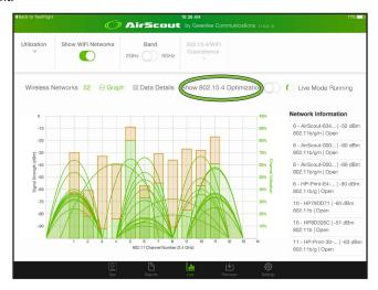
Tapping on the 802.15.4 switch will present a scrollable dropdown that allows selection of a network to improve 802.11 coexistence with 802.15.4.
