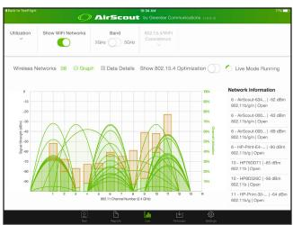
When starting live mode, wireless measurements such as existing network information and channel utilization are immediately collected by the ASM300 from its current location. After a brief period of time, channels supported will be populated with utilization and interference stacked bars as well as WiFi network power and frequency occupancy information.
