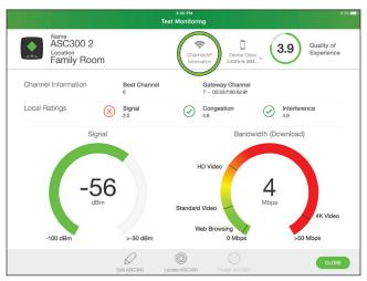
The selected client or master will display all detected Access Points in its location. For gateway tests, the gateway SSID is highlighted in black. AP results can be displayed in graphic or detail formats.
