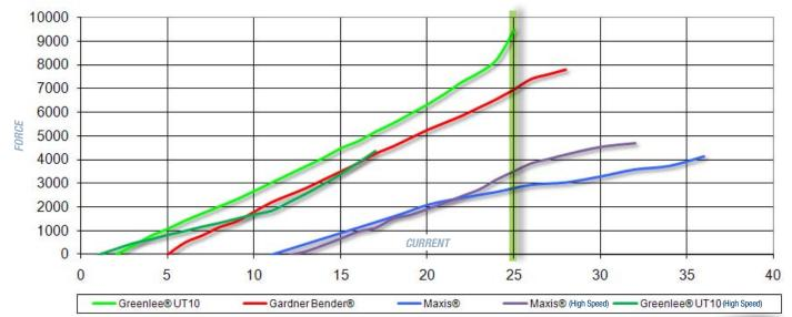
Maxis® and Gardner Bender® units draw more than 25A current at loads greater than 5000 lbs. and 7000 lbs. respectively which can trip the circuit on the job site where the typical circuits are 15A-20A. Greenlee UT10-2S has a circuit breaker which would trip before puller components fail. Maxis® and Gardner Bender® do not have circuit breakers in their units.
