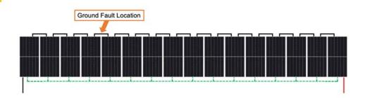
Here's another typical ground fault example with voltage to ground on the negative side.
