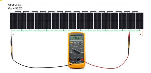
We expected zero volts to ground, but the measurements indicated voltage to ground on the negative sides of the PV string circuit. If we divide both readings to ground by the individual module Voc, we can identify the ground fault location.
