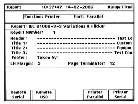
The functions of the soft-keys change as the edit zone is moved through the editable fields of the display using the ▲ ▼ keys; each field is described below. Pressing the VIEW key returns the display to the Report view and allows reports to be printed.
