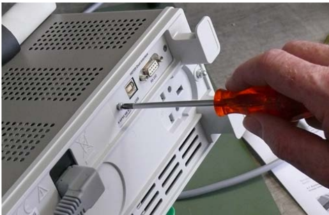
Fig. 2.1: Remove both fastening screws
