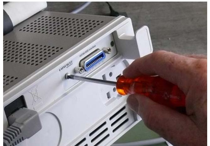
Fig. 2.4: Fit the interface with the previously (Fig. 2.1) removed fastening screws.
