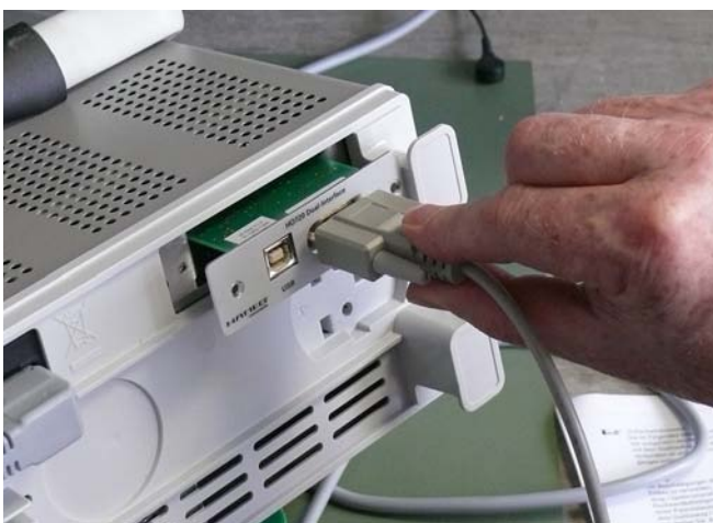
Fig. 2.2: Pull out the interface.
