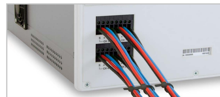
Rear connectors for all channels including SENSE
