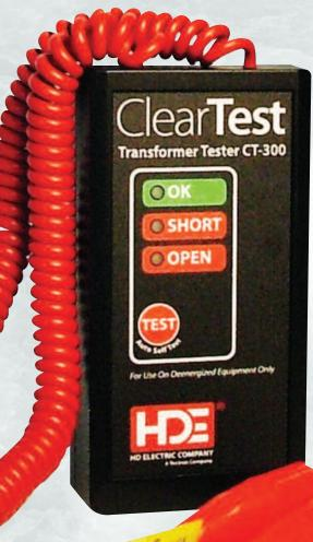
The ClearTest Transformer Tester provides quick and easy tests of de-energized power distribution system transformers. It is a handheld device with a single pushbutton that provides a clear indication of open circuits, short circuits, including shorted turns or shorted windings and confirmation that the test results are OK.
