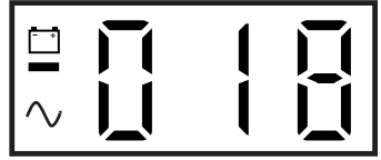
Figure 1 Low battery indicator signal shown in upper lefthand corner of display.
