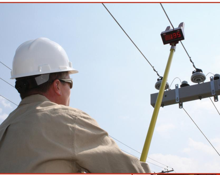
The HVA-2000 is a high voltage digital ammeter designed for taking True RMS AC current measurements up to 2000 amps, 25-500Hz. The HVA can be used on system voltages up to 500kV.
