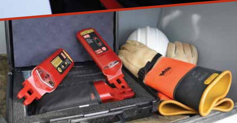
The PRX Proximity Voltage Detectors verify the presence of voltage without contacting the conductor. Three distinct models of testers have been developed for utility professionals:
