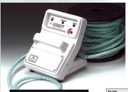
The Hi-Test® Rope Tester is designed to test hot line ropes, slings and straps for dielectric integrity at the time and location they are being used. Ropes with diameters ranging from 3/8 diameter (9.5 mm) to 1-1/2" diameter (38 mm) can be tested along with slings and straps of various sizes.
