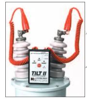
Quick and simple testing of transformers and capacitors for shorts or opens.
