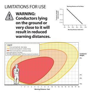
Conductors of different phases in close proximity will also reduce warning distances due to field cancellation effects.
