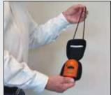
Completely open the zippered case. Test the V-Watch for proper operation before use by pressing and holding the self-test button.
