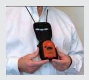
3. Extend the lanyard from the top of the case and place it around the neck. Adjust the lanyard so the V-Watch is worn at mid-chest level.
