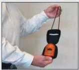
2. Completely open the zippered case. Test the V-Watch for proper operation before use by pressing and holding the self-test button.
