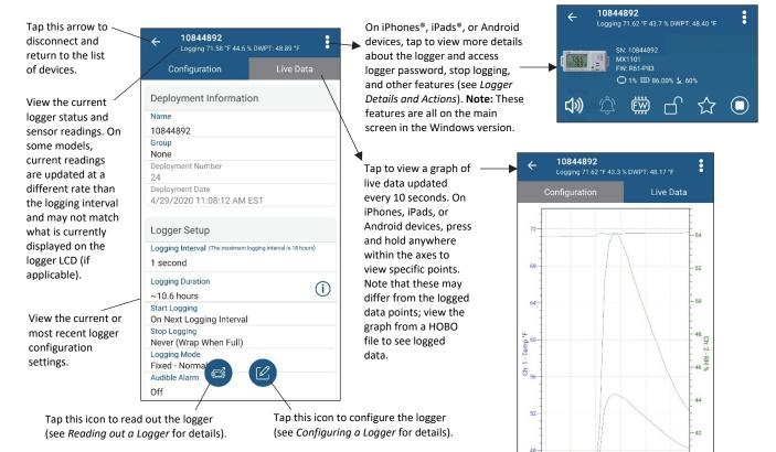
**Note for MX2001 loggers:** When the logger is stopped, the water level reading shown does not reflect any reference water level and water density values you have entered (it reverts to a reference water level of zero and a water density of "Fresh Water adjusted for Temperature"). Once logging begins, the readings shown are then based on the reference water level and water density you entered.
