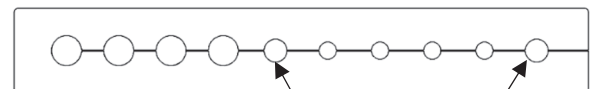
Use one of these two medium holes for the water level sensor cable
