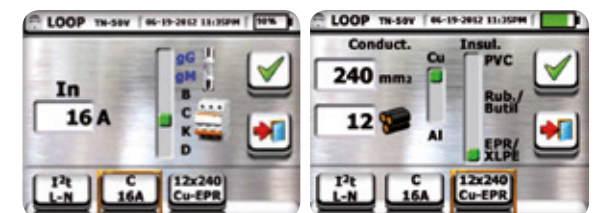
Setting of MCB/fuse type and rated current
