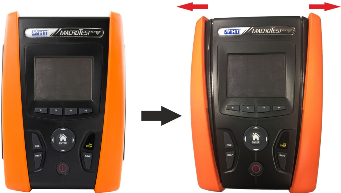
Fig. 40: Remove lateral half-shells
