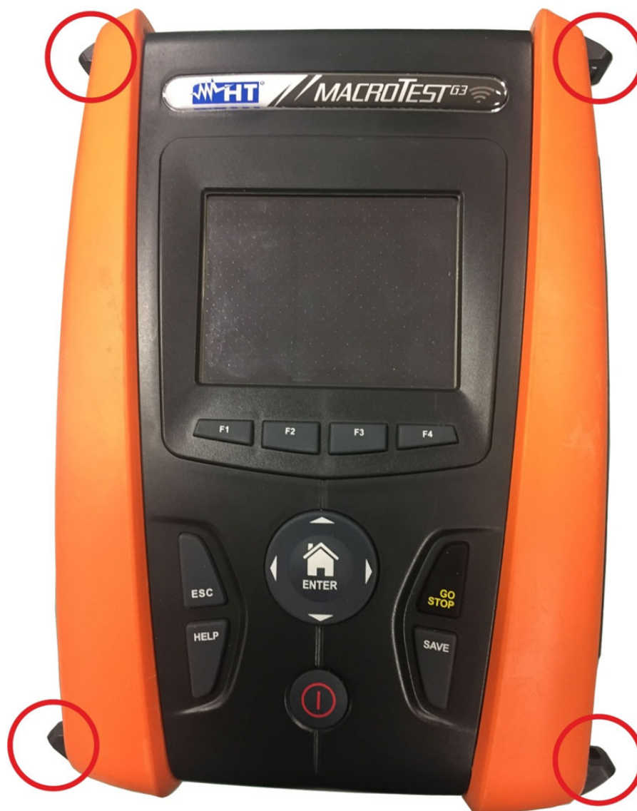
Fig. 42: Instrument with fitted half-shells and hooks
