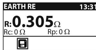
Fig. 26: Result screen of earth resistance measurement
