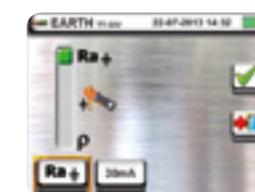
Earth resistance: selection of measurement type
