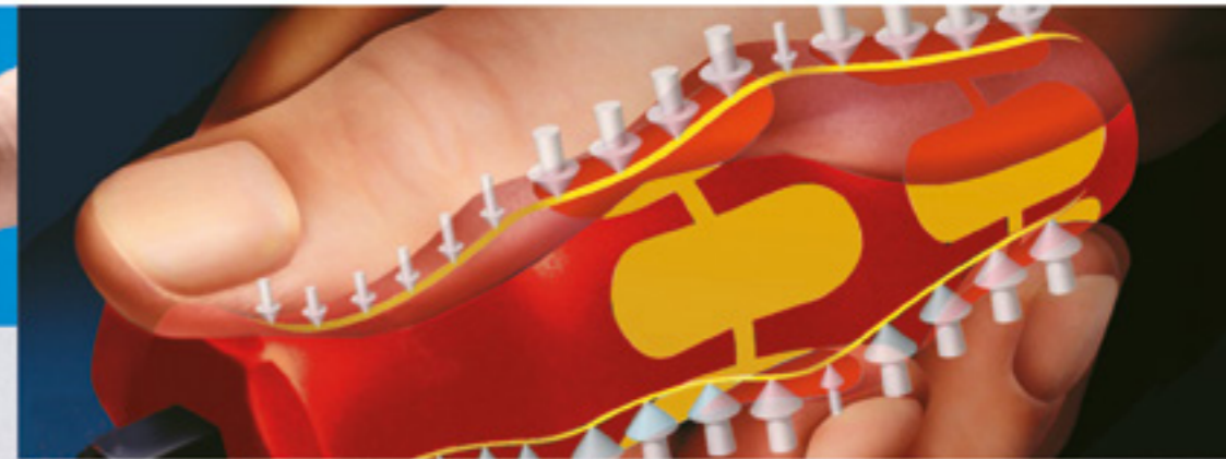
The wide contact surface generates a strong friction with the soft area and guarantees a high transmission of force when gripping.
