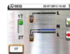
Selection of measurement type of phase sequence
