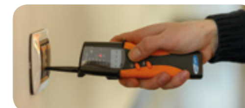
Phase detection function through conductive button.
