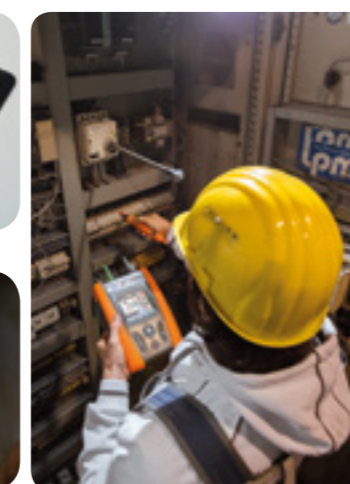
Start/stop measuring with remote lead PR400.
