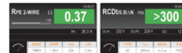
2-wire continuity test
