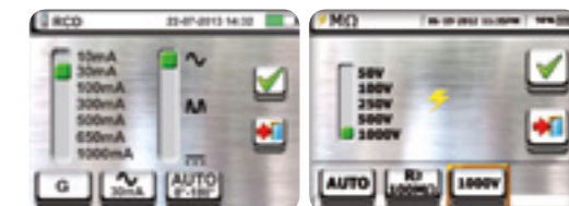
Selection of RCD type and tripping current
