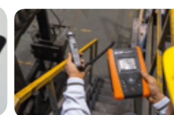
Lux measurement with accessory HT53/05.
