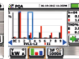
Power measurement: harmonics
