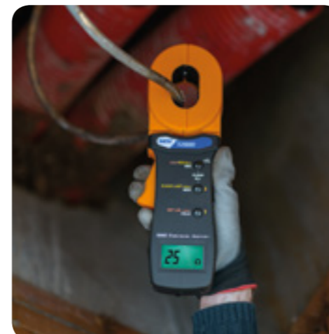
Measurement of earth resistance with Clamp T2100.
