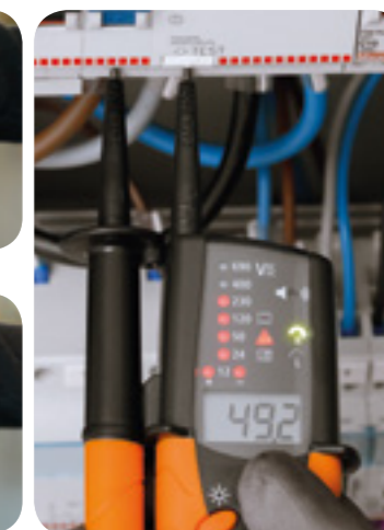
Measurement of phase sequence.
