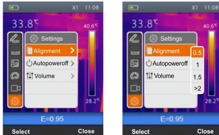
Fig. 13: Setting the alignment distance
