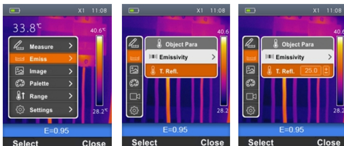
Fig. 18: Setting the Reflected Temperature on the instrument
