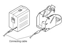
When using the sleep function, insert one end of the connecting cable into the jack at the back of the iron holder and the other end into the jack at the back of the soldering station to connect them.
