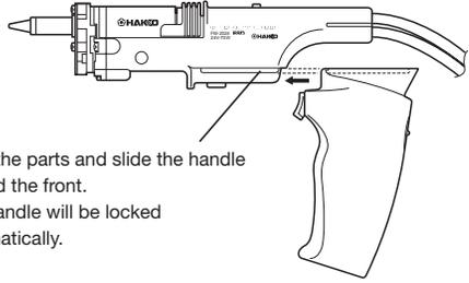
Align the parts and slide the handle toward the front. The handle will be locked automatically.
