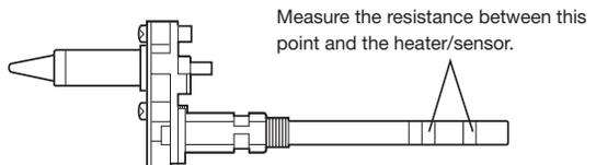
Measure the resistance at room temperature (15 to 25°C ; 59 to 77°F). The normal range is  $8\Omega \pm 10\%$ . If the resistance is outside this range, replace the nozzle assembly.
