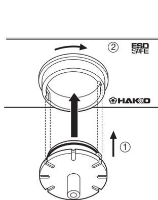
After replacing the ceramic paper filter (DCB), press the filter case cover with its tabs inserted into the corresponding slots in the filter case then turn clockwise to lock it.
