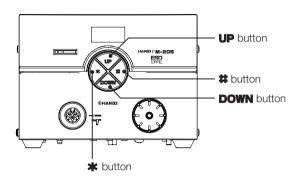
The front panel of the HAKKO FM-205 has four controls.
