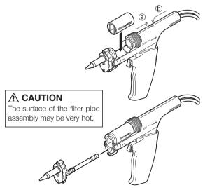
Attaching and replacing the nozzle cartridge Insert the nozzle cartridge fully into the grip as shown in the illustration. Once the nozzle cartridge is inserted, it is locked automatically.
