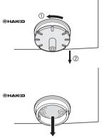
The filter is clogged with hardened flux.
