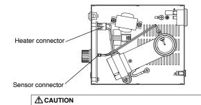
Measure the resistances of the heater and the sensor when their temperatures are at room temperature.
