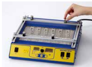
Adjust screws to match board width and length.
