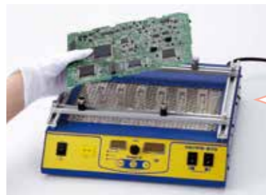
Boards are hot after operation and must be handled with care.
