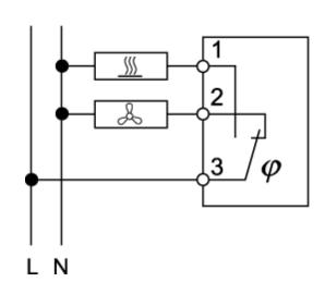
· Mechanical Humidistat regulates the control of heaters or fans whenever the preset level
