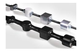
High shrink-ratio heavy-duty heat shrinkable tubing designed to pass over large size connectors and shrink down onto much smaller cable jackets. The thermoplastic adhesive lined tubing provides environmental sealing, excellent insulation and resistance to impact and abrasion.
