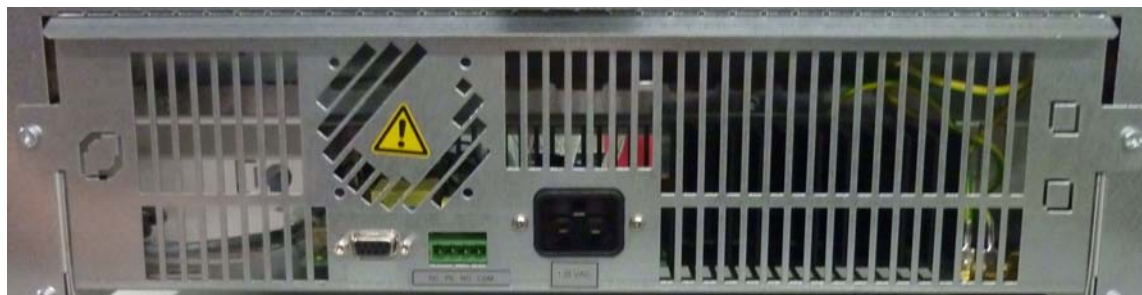
Figure 5-9 AC Power Supply Socket
