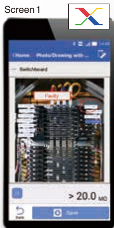
Take a picture of the test location and map measured values on it
