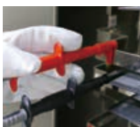
For clamping around the target busbar
