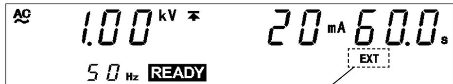
When  $\overline{\text{EXT-E}}$  of the external I/O terminal is at LOW level, EXT lights up when the REMOTE CONTROL BOX is active.
