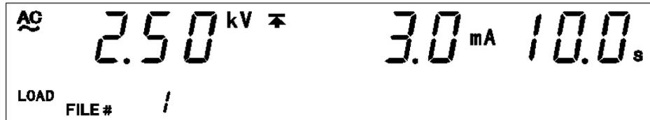
3. Execute file loading by pressing the **ENTER** key. The selected file will be loaded, and the program-mode window will be displayed. To cancel loading, press the **STOP** key. The unit will change to the program mode with the file number used or loaded previously.
