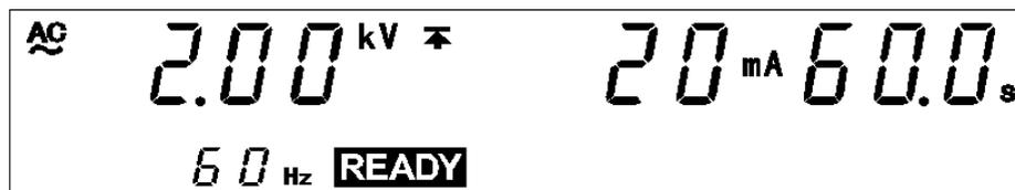
To abort the save procedure, press the **STOP** key at Step (4). The unit halts the save procedure and reverts to the READY state.
