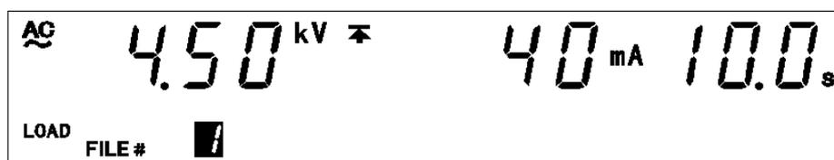
At this time, the "test frequency" (in the case of AC-withstand-voltage) can be confirmed using the ◀ key, the "lower-limit value" can be confirmed using the ▶ key, and the "ramp-up/down time" can be confirmed using the ON/OFF key.
