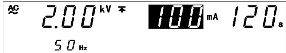
In this example, switch from **100 mA** to **20 mA** using the  $\blacktriangledown/\blacktriangle$  keys.
