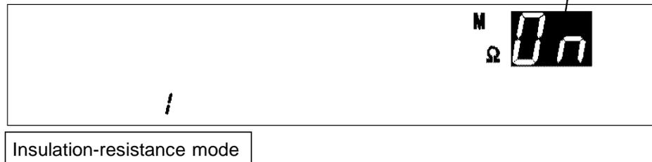
10. When the **ENTER** key is pressed, the **DATA INPUT** lamp lights up. Set the withstand-voltage or insulation-resistance test conditions in the step being set. For the setting items, see Test setting conditions in Chapters 3 and 4.
