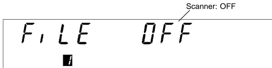
3. To use the scanner, select the mode.\* When the scanner is not used, set it to OFF. (\* **↕**: single scan; **↕↕**: multi-scan)
