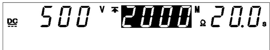
The upper-limit value is set at 2000 MΩ. Turn it **OFF**, as it is not needed. To change to **OFF**, press the **ON/OFF** key.
