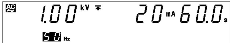
Test-voltage type: **AC 50 Hz**
