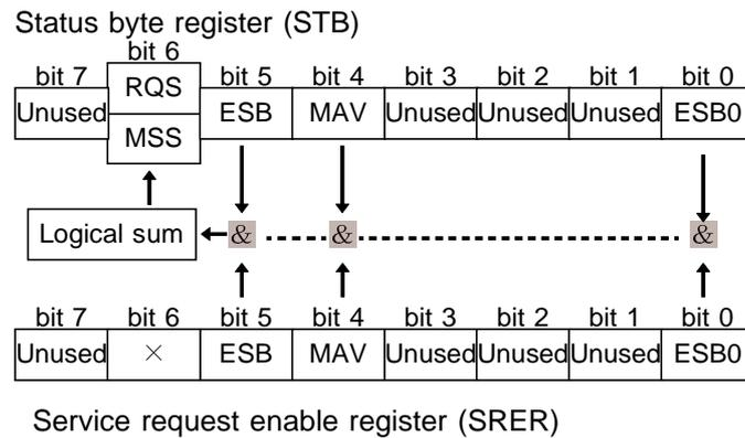
The RQS bit is synchronized with service requests, and is read out and simultaneously cleared when serial polling is being performed. Although the MSS bit is only read out on an \*STB? query, on a \*CLS command for example it is not cleared until the event is cleared.
