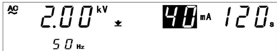
The lower-limit value is set at **40 mA**. Turn it OFF, as it is not needed. To change to **OFF**, press the **ON/OFF** key.
