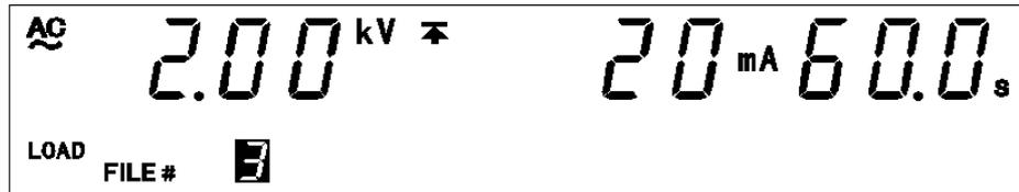
3. The "test voltage" and "test frequency" (in the case of AC-withstand-voltage) can be confirmed using the **◀** key, the "upper-limit value" and "lower-limit value" can be confirmed using the **▶** key, and the "test time" and "ramp-up/down time" can be confirmed using the **ON/OFF** key.
