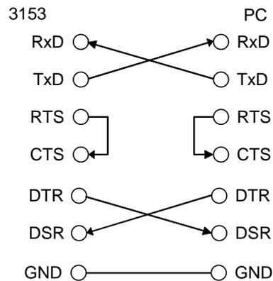
Connector on cable side: D-Sub 9 Pin female
