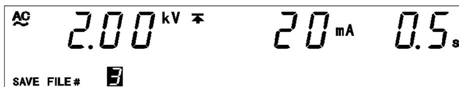
4. The "test voltage" and "test frequency" can be confirmed using the **◀** key, the "upper-limit value" and "lower-limit value" can be confirmed using the **▶** key, and the "test time" and "ramp-up/down time" can be confirmed using the **ON/OFF** key.
