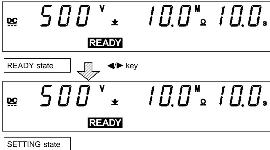
1. In the insulation-resistance mode READY state, when you press the ◀▶ keys, the flashing cursor appears where the test-voltage is indicated to show that the unit is in the SETTING state. (The **READY** light goes out and tests cannot start even if the **START** key is pressed.)
