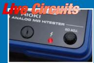
The LIVE CIRCUIT LED will light up in red whenever the voltage exceeds 20V AC between the LINE and EARTH terminals, and when at least 20V DC is still remaining during the auto discharge.
