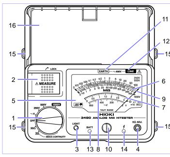
1. Function switch: Select measurement functions
