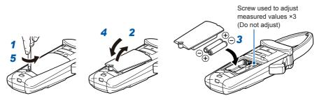
Do not adjust any screws other than the screw holding the battery cover in place. Do not adjust the three screws underneath the cover, which are used to adjust measured values, as doing so may prevent accurate measurement.
