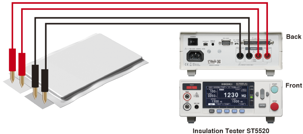
Figure 13. Insulation Tester ST5520 to measure the insulation resistance of battery cells
