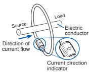
Clamp only the conductor you wish to measure with the current direction indicator pointing toward the load side. (To ensure that the measured current and sensor output have the same phase.)
