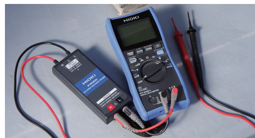
Fig. 2. The DT4261 and P2000 being used together.
