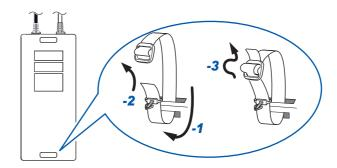
Attach the strap buckle to a compatible instrument and connect it to the clip that you attached to the device with the strap.
