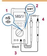
The open terminal voltage is approx. 2.5 V or less. The measurement current (DC) is approx. 96 nA. (p. 85) To avoid damage to the measurement object, check the specifications before use.
