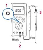
The open terminal voltage is approx. 2.5 V or less. The measurement current (DC) varies depending on the range. (p. 84) To avoid damage to the measurement object, check the specifications before use.
