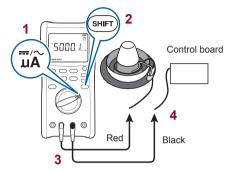
Example: Measuring the current of the burner flame (µA)
