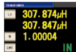
Transformer measurement mode Turn ratio measurement and judgment screen
