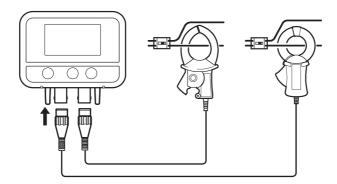
Prepare the combination of Display Unit CM7290 and Output Cord L9095 or that of Display Unit CM7291 and Output Cord L9095 when you use one of the following clamp sensors: Models CT7631, CT7636, CT7642, CT7731, CT7736, CT7742, CT7044, CT7045, and CT7046.
