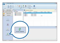
If the software version is older than 1.20, a communication error (protocol error) occurs in any communications attempted between the instrument and Wireless Logger Collector.
