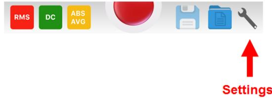
Once in settings, you will have the ability to change the LED color display of the wireless module that you are connected to, and the SSID display name of the device. When either of these are changed, the app will need to reboot and reconnect to the wireless module. So after the app closes, it will direct you to the iPhone WiFi settings, where you can reconnect to the new SSID name or color, and then open the app again.
