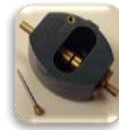
Test Cell: TCDE ASTM D877 (pictured left)
