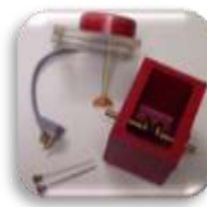
Test Cell: TCVDE ASTM D1816 (pictured left)
