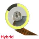
Hybrid light engines use a combination of LEDs and lasers for the red and blue light channels. Green lasers are still too expensive and green LEDs are not bright enough, so to create green these hybrids use a phosphor disk. That process is detailed below.
