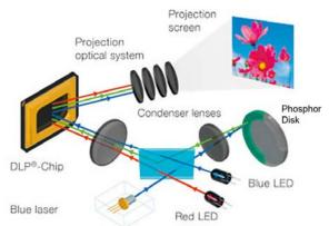
It's key to point out that the phosphor disk will degrade over time. This technology is new to projection... so the industry is still learning about the long-term life span of the phosphor.
